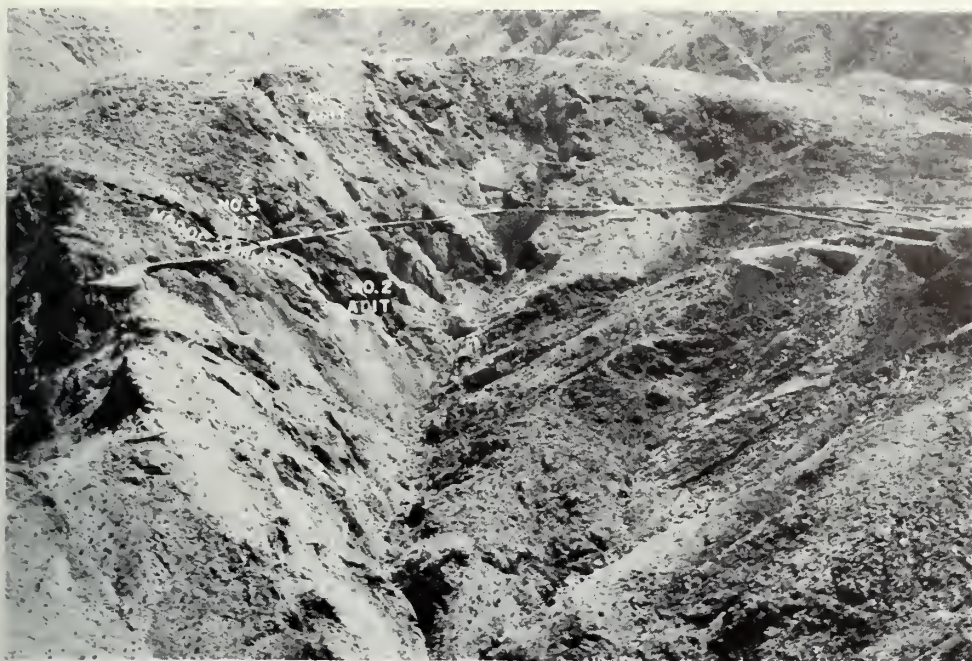
Photo 11. Aerial view southwest toward the upper workings of the Modoc mine. The Modoc thrust passes through the portals of the No. 2 and No. 3 adits, and much of the mineralization is in the footwall of it.
